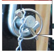
Lynch Pin fitted correctly
